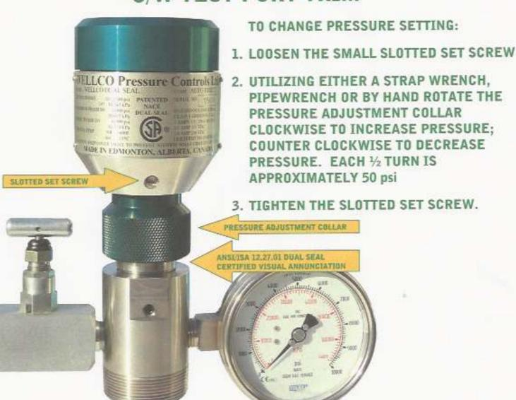
INSTALL CONTROL WITH EITHER PIPEWRENCH OR FLAT WRENCH ONTO A LOCKING BALL VALVE TO UTILIZE THE TEST PORTS ON THE TRIM
